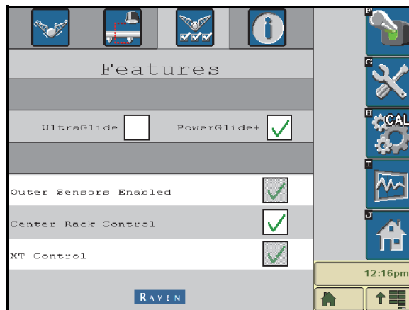
FIGURE 19. ISO Terminal Programmed to Run in PowerGlide Plus Mode
