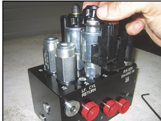
FIGURE 18. Coil Reinstalled on the AutoBoom Valve
