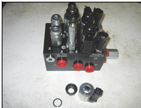
FIGURE 14. Coil Removed from the AutoBoom Valve
