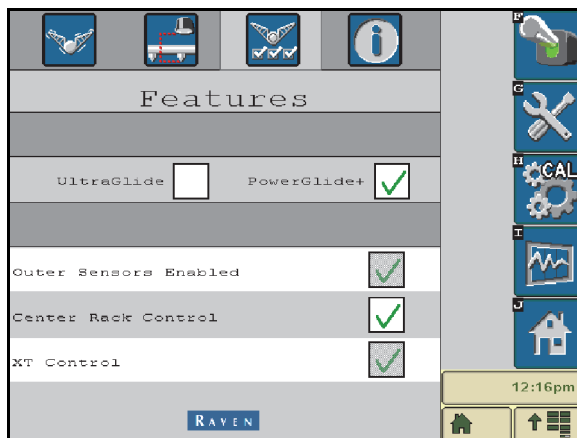
FIGURE 12. ISO Terminal Programmed to Run in PowerGlide Plus Mode
