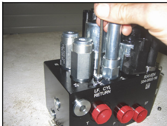
FIGURE 17. Port Plug Reinstalled on the AutoBoom Valve
