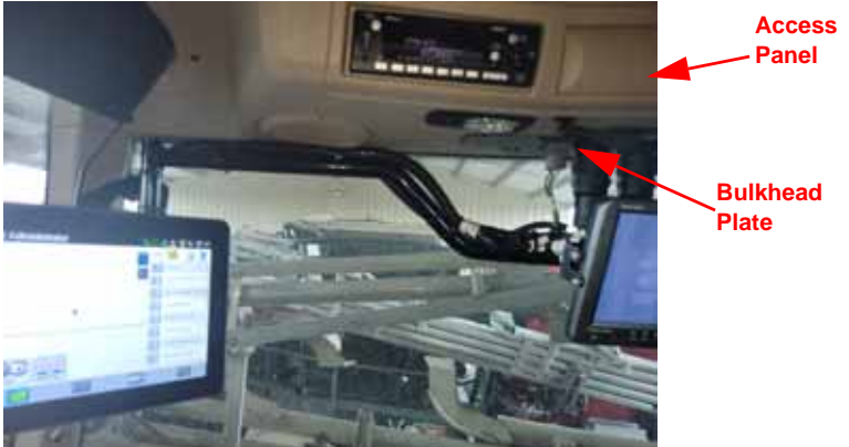
FIGURE 9. Access Cover and Bulkhead Plate
