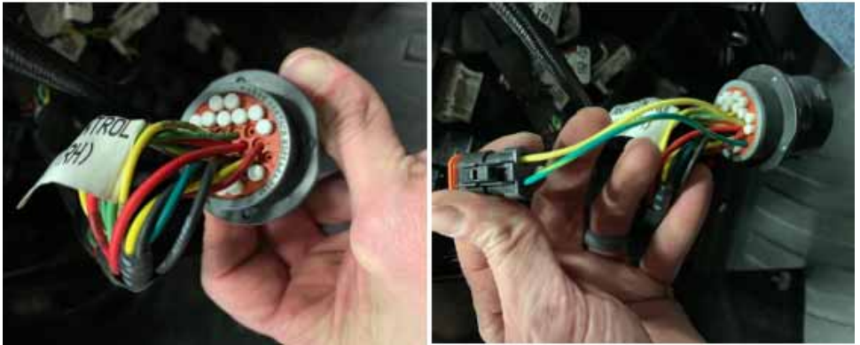
FIGURE 6. Raven Vehicle CAN Cable Installed in Bulkhead
