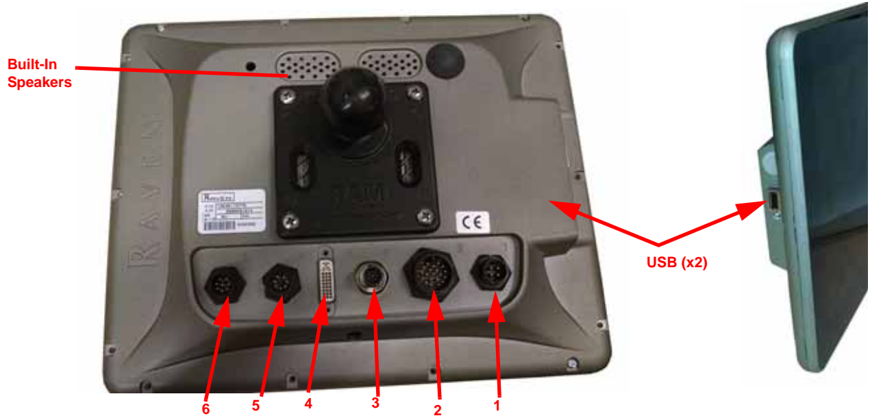
FIGURE 5. Viper 4+ Ports and Connectors
