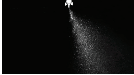
Unique angle of incline specifically engineered to maximize droplet deposition on vertical targets.
