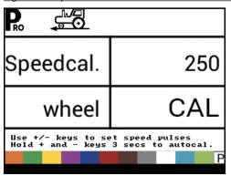
NOTE: When the Automatic Calibration Mode is activated, no other functions are possible until the console receives Pulses for calibration. To deactivate the Automatic Calibration Mode, press the PLUS button until a number is displayed.
