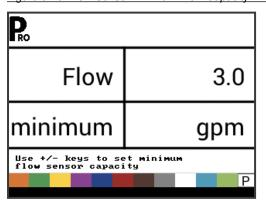
Minimum flow capacity can be located in the flow meter manufacturer's literature.
