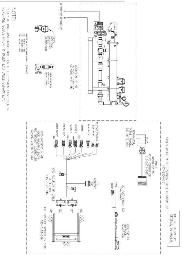
FIGURE 7. ISOBUS AccuFlow HP (3 Section Bar)
