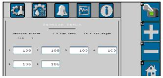
NOTE: Section measurements should be programmed into the VT display using the same units (e.g. inches, centimeters) selected in the options or settings on the VT display. Refer to the operation manual for the specific VT display to configure the display units.
