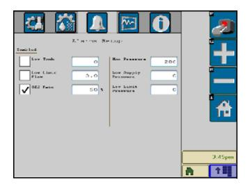
If any of these alarm conditions is detected by the product control node, the corresponding alert will be displayed on the VT display and allow the operator to respond to the condition before resuming application.
