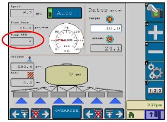
The current pump RPM is displayed in this area when a Pump RPM Cal value is entered. Refer to *Pump RPM Cal* section on page 22 to set the Pump RPM Cal value.
