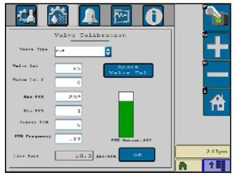
NOTE: To accept the currently displayed settings, or once settings have been adjusted properly, select the "OK" button in the lower right corner of the display to return to the Product Calibration display.
