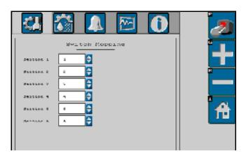
NOTE: Switch mapping is only available if an optional Raven ISO Switch Box is detected on the ISOBUS.
