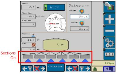
Below the tank volume display, the status of each configured section is displayed.
