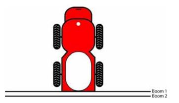
NOTE: Specialized plumbing, cabling, and a relay box are required to utilize a tiered boom configuration. Generally, sprayers are not set up for this feature from the factory.
