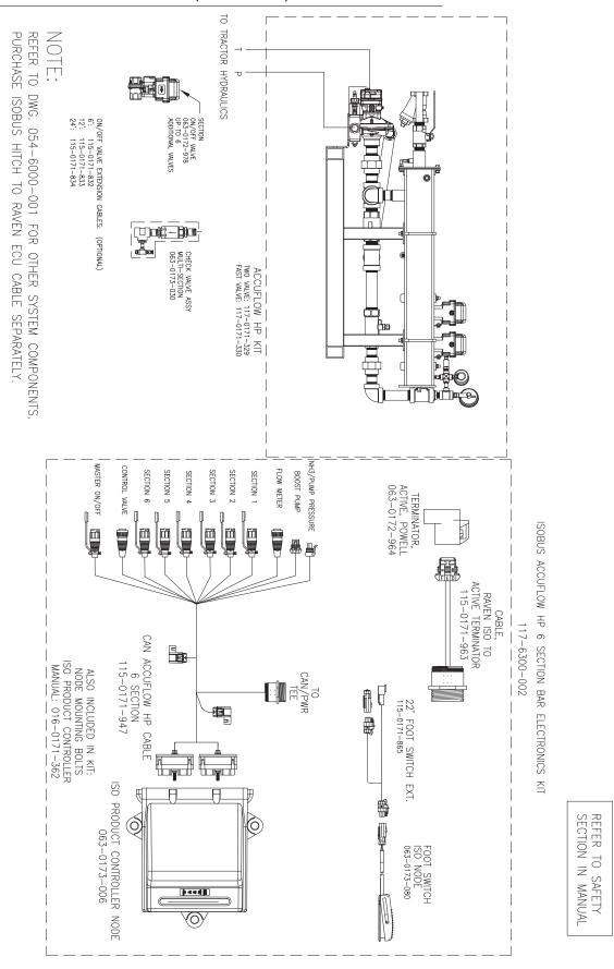
FIGURE 9. ISOBUS AccuFlow HP (6 Section Bar)
