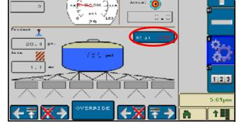
Touch this button to toggle the selected ISO injection pump on or off.
