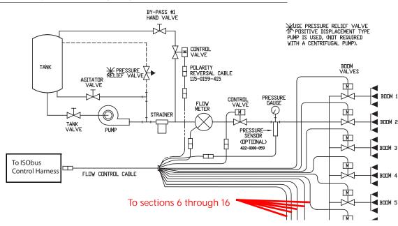
FIGURE 2. By-Pass Plumbing Diagram
